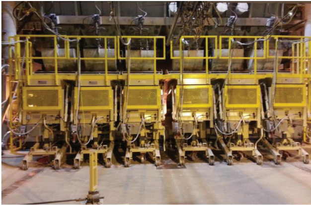
► The streamlined design of the modular charger allows for a tight fit on the sides. All adjustments are made from the rear of the unit.
